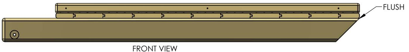
3: ATTACH USING #8 X 1-1/2" WOOD SCREWS THROUGH THE PRE-DRILLED HOLES INTO THE ROOF SUPPORT.
