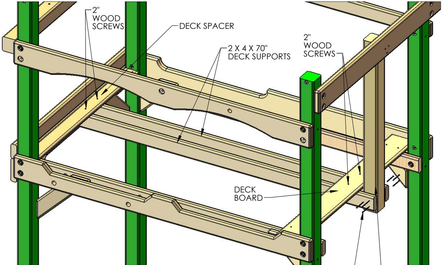
HAVE AN ASSISTANT HOLD THE END OF THE DECK SUPPORTS WHILE YOU PUT IN SCREWS THROUGH DECK BOARD AND DECK SPACER.
