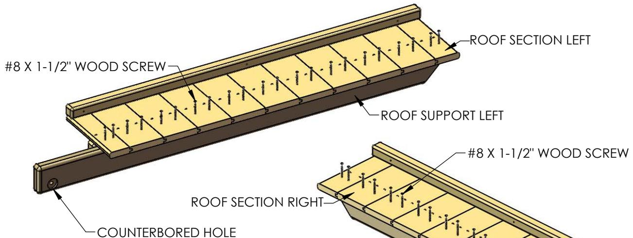
4: FIND THE 2 X 4 X 51.13" ROOF SUPPORT RIGHT AND THE 4 X 10 X 43.50" ROOF PANEL RIGHT ASSEMBLY. REPEAT SUB STEP 1 - 3 FOR THE ROOF SECTION RIGHT.
