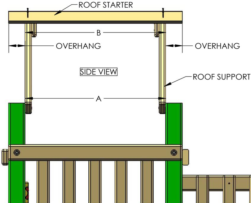
BEFORE INSTALLING THE ROOF STARTERS MAKE SURE DIMENSIONS A AND B MATCH. ALSO MAINTAIN THE SAME OVERHANG OF THE ROOF STARTERS ON EACH SIDE OF THE ROOF SUPPORTS.
