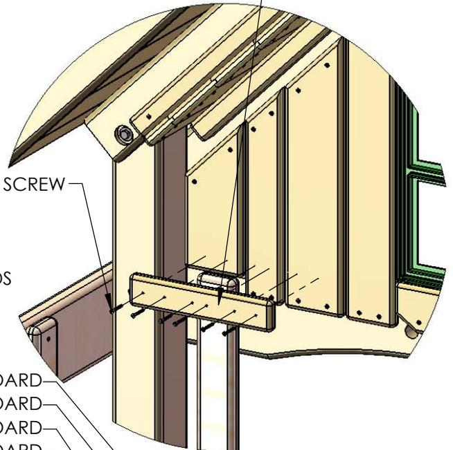
4: MOUNT THE 1 X 2 X 9.88" WALL PANEL BOARD CENTERED ON TOP OF THE PREVIOUS WALL PANEL BOARDS. IT SHOULD BE ABOVE THE PLAY SET PANEL SLAT AS SHOWN IN THE DIAGRAM. MAKE SURE THE HOLES ARE CENTERED ON EACH OF THE BOARDS AND FASTEN IT USING SIX #8 X 1-1/4" WOOD SCREWS.
