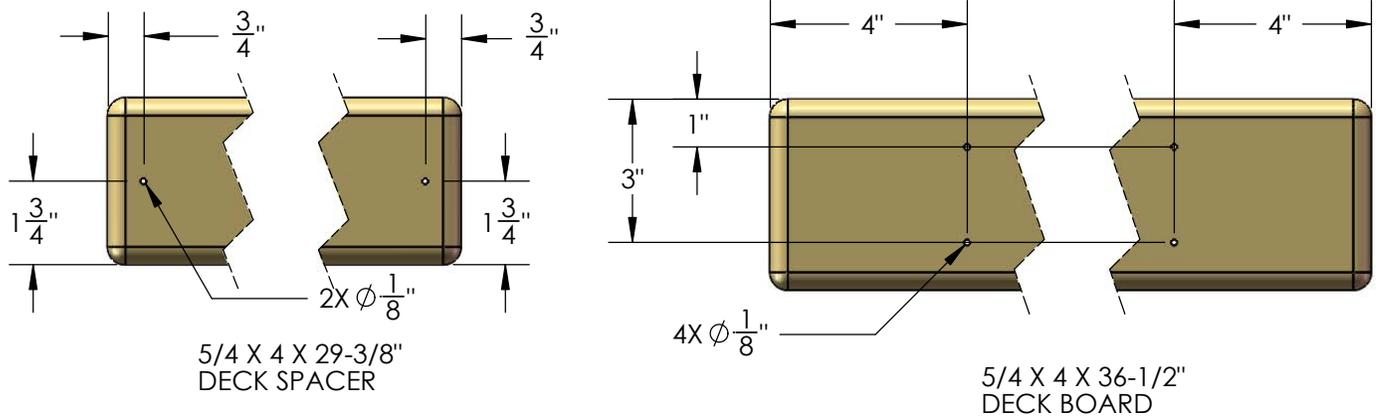
2: PLACE THE 5/4 X 4 X 29-3/8" DECK SPACERS BETWEEN THE CORNER POSTS. MAKE EACH DECK SPACER FLUSH TO THE INSIDE SURFACE OF THE 2 X 6 OR THE OUTSIDE SURFACE OF THE CORNER POSTS. DO NOT ATTACH THE DECK SPACERS YET.
