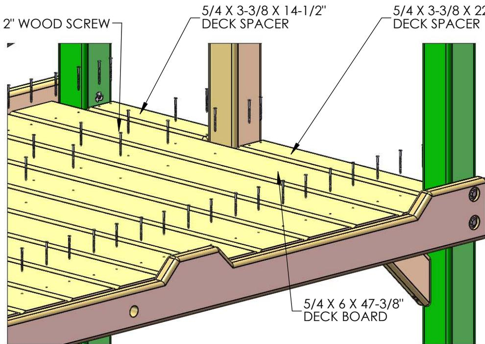
2: START WITH A 5/4 X 6 X 47-3/8" DECK BOARD AT ONE END OF THE FORT. CENTER THE BOARD BETWEEN THE FRONT FACE BOARD AND THE REAR BOTTOM PANEL BOARD AND ATTACH IT WITH 2" WOOD SCREWS THROUGH THE PREDRILED HOLES AND INTO THE DECK SUPPORT BELOW. LEAVE A UNIFORM (APPROX. 1/4") SPACE BETWEEN THE DECK BOARDS. NOTE: THE TOP OF THE SCREW HEAD SHOULD BE FLUSH TO THE TOP OF THE DECK BOARDS.
