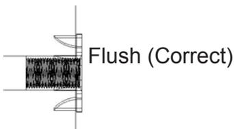
Cross Section end view, you are looking at an X-ray view of the post and T-nut. The barrel of the T-nut is in the corner post the line is the face of the wood.
