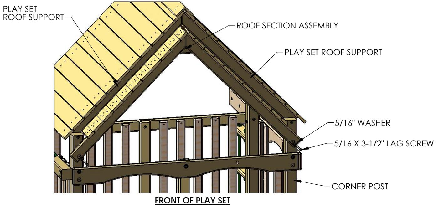
3: FASTEN THE ROOF SECTION TO THE PLAY SET ROOF SUPPORTS USING SIX #8 X 2-1/2" WOOD SCREWS THROUGH THE TOP BATTEN PRE-DRILLED HOLES.
