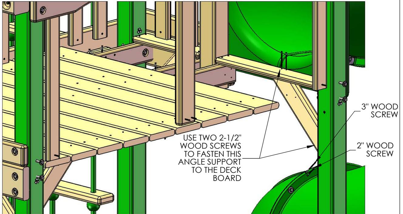
3: FOR THE 2 X 4 X 18" ANGLE SUPPORTS AT THE RIGHT FRONT USE TWO 2-1/2" WOOD SCREWS THROUGH THE DECK AND INTO THE ANGLE SUPPORT. USE ONE 2" AND ONE 3" WOOD SCREW TO FASTEN THE RIGHT FRONT ANGLE SUPPORTS TO THE RIGHT FRONT CORNER POST.
