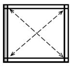
The diagonal measurements should be the same from corner post to corner post. If not, adjust corner posts so that the distance is equal.
