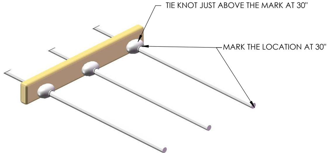
4: MEASURE 19" FROM THE TOP OF THE ROPE LADDER RUNG ON THE ROPE AND MARK THIS LOCATION. MAKE SURE THE BOARD IS RESTING AGAINST THE PREVIOUS KNOT THAT WAS TIED WHEN MEASURING.
