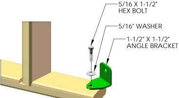
7: INSTALL THE 1-1/2" X 1-1/2" ANGLE BRACKETS TO THE INSIDE OF THE LADDER RAILS WITH 5/16 X 1-1/2" BOLTS, 5/16 WASHERS, INTO THE 5/16" T-NUTS.
