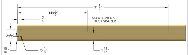
2: START WITH THE 5/4 X 3-3/8 X 63" DECK SPACER AT ONE END OF THE FORT. CENTER THE BOARD BETWEEN THE CORNER POSTS AND ATTACH IT WITH 2" WOOD SCREWS THROUGH THE PREDRILED HOLES AND INTO THE DECK SUPPORT BELOW. NOTE: THE TOP OF THE SCREW HEAD SHOULD BE FLUSH TO THE TOP OF THE DECK SPACER.
