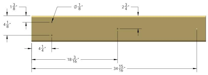
2: START WITH A 5/4 X 6 X 69-7/8" DECK BOARD AT ONE END OF THE FORT. CENTER THE BOARD BETWEEN THE FRONT FACE BOARD AND THE REAR BOTTOM PANEL BOARD AND ATTACH IT WITH 2" WOOD SCREWS THROUGH THE PREDRILED HOLES AND INTO THE DECK SUPPORT BELOW. LEAVE A UNIFORM (APPROX. 1/4") SPACE BETWEEN THE DECK BOARDS. NOTE: THE TOP OF THE SCREW HEAD SHOULD BE FLUSH TO THE TOP OF THE DECK BOARDS.
