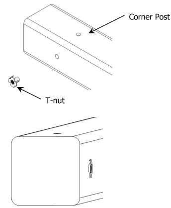
This picture shows the T-nut insert and installed flush to the wood.
