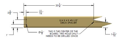
2: PLACE THE 5/4 X 4 X 40-1/2" DECK SPACER AT ONE END OF THE FORT. CENTER THE BOARD BETWEEN THE CORNER POSTS AND ATTACH IT WITH 2" WOOD SCREWS THROUGH THE PRE-DRILLED HOLES INTO THE DECK SUPPORT BELOW. NOTE THE TOP OF EACH SCREW HEAD SHOULD BE FLUSH TO THE TOP OF THE DECK SPACER.
