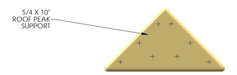
2: PLACE THE 5/4 X 10" ROOF PEAK SUPPORT AGAINST THE ANGLED ROOF SUPPORTS AND FLUSH TO THE SIDES OF THE ANGLED ROOF SUPPORTS. FASTEN THE ROOF PEAK SUPPORT TO THE ANGLED ROOF SUPPORTS WITH 1-1/2" WOOD SCREWS. REPEAT ON OTHER SIDE.
