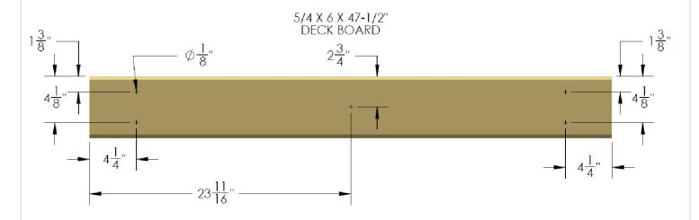
2: START WITH A 5/4 X 6 X 47-1/2" DECK BOARD AT ONE END OF THE FORT. CENTER THE BOARD BETWEEN THE FRONT FACE BOARD AND THE REAR BOTTOM PANEL BOARD AND ATTACH IT WITH 2" WOOD SCREWS THROUGH THE PREDRILLED HOLES AND INTO THE DECK SUPPORT SHOWN BELOW. LEAVE A UNIFORM (APPROXIMATELY 1/4") SPACE BETWEEN THE DECK BOARDS. NOTE THE TOP OF THE SCREW HEAD SHOULD BE FLUSH TO THE TOP OF THE DECK BOARDS.
