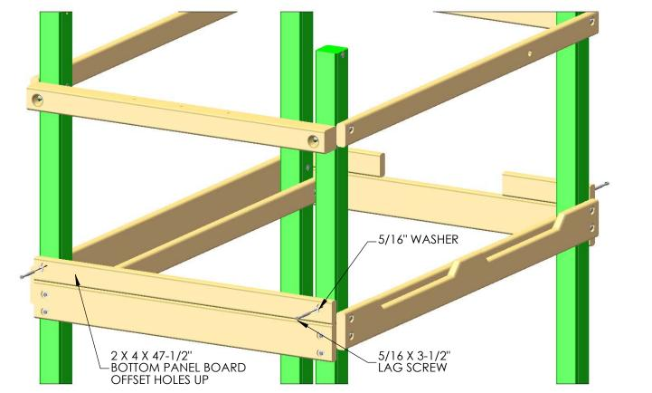
2: PLACE THE 2 X 4 X 14" BOTTOM PANEL BOARD ON TOP OF THE 2 X 6 PANEL BOARD, AND FASTEN TO THE CORNER POSTS WITH 5/16 X 3-1/2" LAG SCREWS WITH 5/16" WASHERS.
