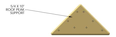
2: PLACE THE 5/4 X 10" ROOF PEAK SUPPORT AGAINST THE ANGLED ROOF SUPPORTS FLUSH TO THE SIDES. FASTEN THE ROOF PEAK SUPPORT TO THE ANGLED ROOF SUPPORTS WITH 1-1/2" WOOD SCREWS
