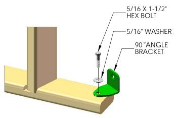
7: INSTALL THE 90° ANGLE BRACKETS TO THE INSIDE OF THE LADDER RAILS WITH 5/16 X 1-1/2" BOLTS, 5/16 WASHERS, INTO THE 5/16" T-NUTS.
