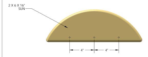
2: PLACE THE 2 X 6 X 16" SUN CENTERED AGAINST THE 5/4 X 2-5/8 X 42" SUN SUPPORT. FASTEN THE SUN TO THE SUN SUPPORT WITH 2" WOOD SCREWS.
