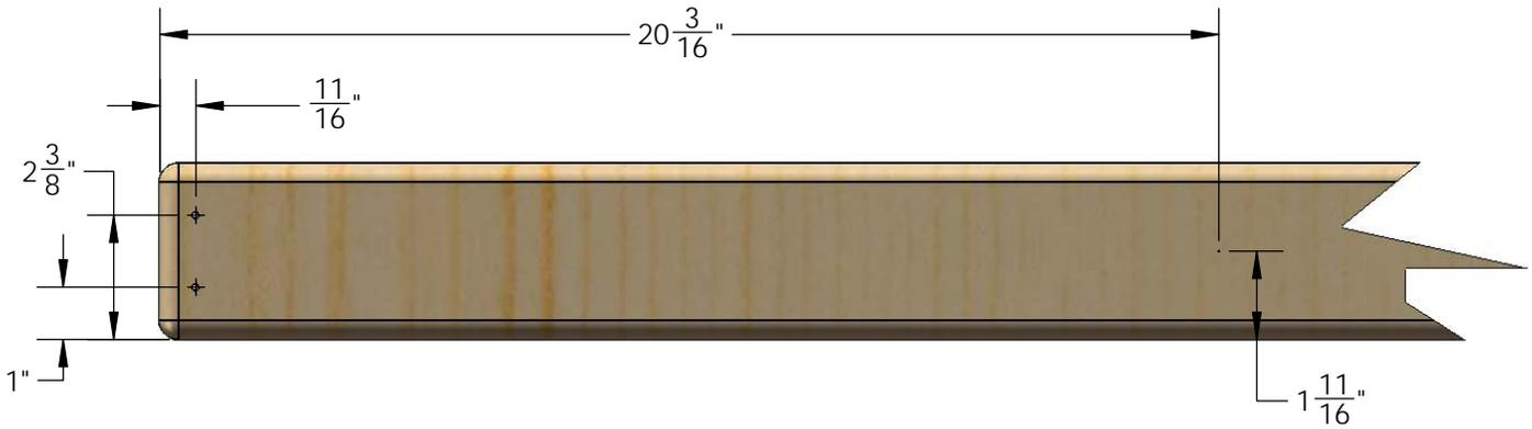
2: PLACE THE 5/4 X 4 X 40-3/8" DECK SPACER AT ONE END OF THE FORT. CENTER THE BOARD BETWEEN THE CORNER POSTS AND ATTACH IT WITH 2" WOOD SCREWS THROUGH THE PREDRILLED HOLES AND INTO THE DECK SUPPORT BELOW. NOTE THE TOP OF THE SCREW HEAD SHOULD BE FLUSH TO THE TOP OF THE DECK SPACER.
