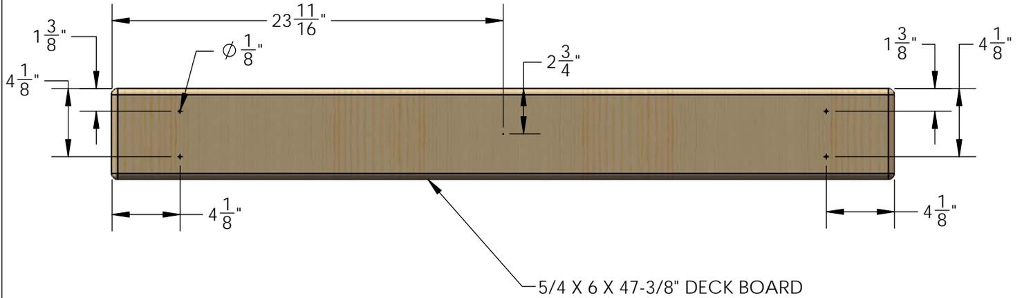
2: START WITH A 5/4 X 6 X 47-3/8" DECK BOARD AT ONE END OF THE FORT. CENTER THE BOARD BETWEEN THE FRONT FACE BOARD AND THE REAR BOTTOM PANEL BOARD AND ATTACH IT WITH 2" WOOD SCREWS THROUGH THE PREDRILLED HOLES AND INTO THE DECK SUPPORT BELOW. LEAVE A UNIFORM (APPROX. 1/4") SPACE BETWEEN THE DECK BOARDS. NOTE: THE TOP OF THE SCREW HEAD SHOULD BE FLUSH TO THE TOP OF THE DECK BOARDS.
