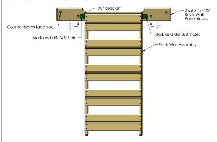
3: Now flip the Rock Wall Panel Board over and install a T-nut into each of the holes you just drilled. Place the Rock Wall Panel Board and the Rock wall aside for use in a later step.
