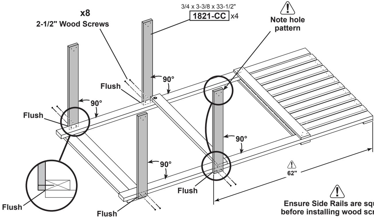
Ensure Side Rails are square before installing wood screws.
