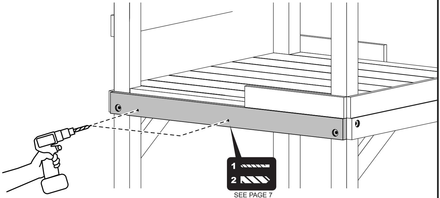
Pre-drill two 1/4" pilot holes at marked locations.
