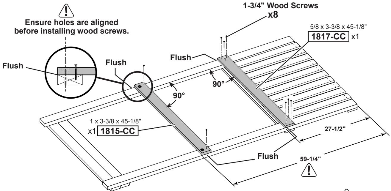
Ensure Side Rails are square before installing fasteners.
