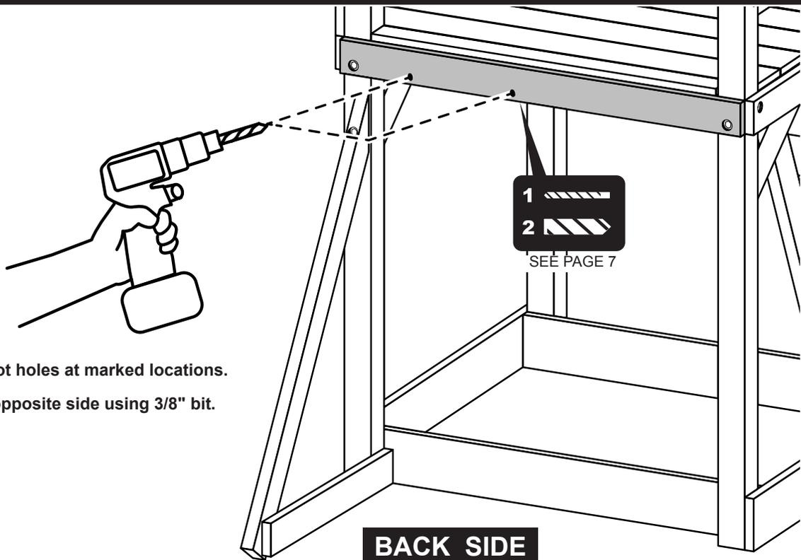
Pre-drill two 1/4" pilot holes at marked locations.
