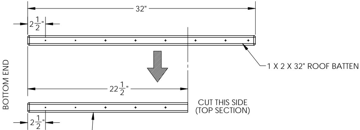
3: ONCE THE ROOF BATTEN HAS BEEN CUT TO 22-1/2", PLACE IT AGAINST THE REAR ROOF PANEL. THE UNFINISHED END (TOP END) MUST BE POINTING TOWARDS THE ROOF PEAK, AND THE BOTTOM END MUST BE FLUSH TO THE BOTTOM EDGE OF THE ROOF FINISHER. INSERT 1-1/4" WOOD SCREWS THROUGH THE PRE-DRILLED HOLES ALONG THE BATTEN.
