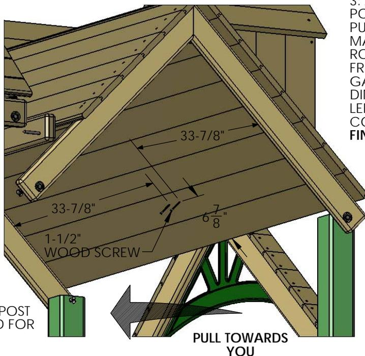
3: AFTER THE GABLE ASSEMBLY IS IN ITS FINAL POSITION. GO INSIDE ON TOP OF THE DECK AND PULL THE GABLE ASSEMBLY TOWARDS YOU MAKING SURE IT IS FLUSH TO THE OUTSIDE OF THE ROOF AND INSERT TWO 1-1/2" WOOD SCREW FROM UNDERNEATH THE ROOF INTO THE GABLE ASSEMBLY ROOF PEAK. USE THE DIMENSIONS SHOWN IN THE DIAGRAM TO THE LEFT TO INSERT THE WOOD SCREWS IN THE CORRECT LOCATION. **REMOVE THE ROOF FINISHERS, THESE WILL BE USED IN A LATER STEP.**
