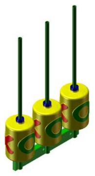
3: Locate the green Bracket and place on top of assembly. Line up the holes in the bracket with the Dowels on the unit.
