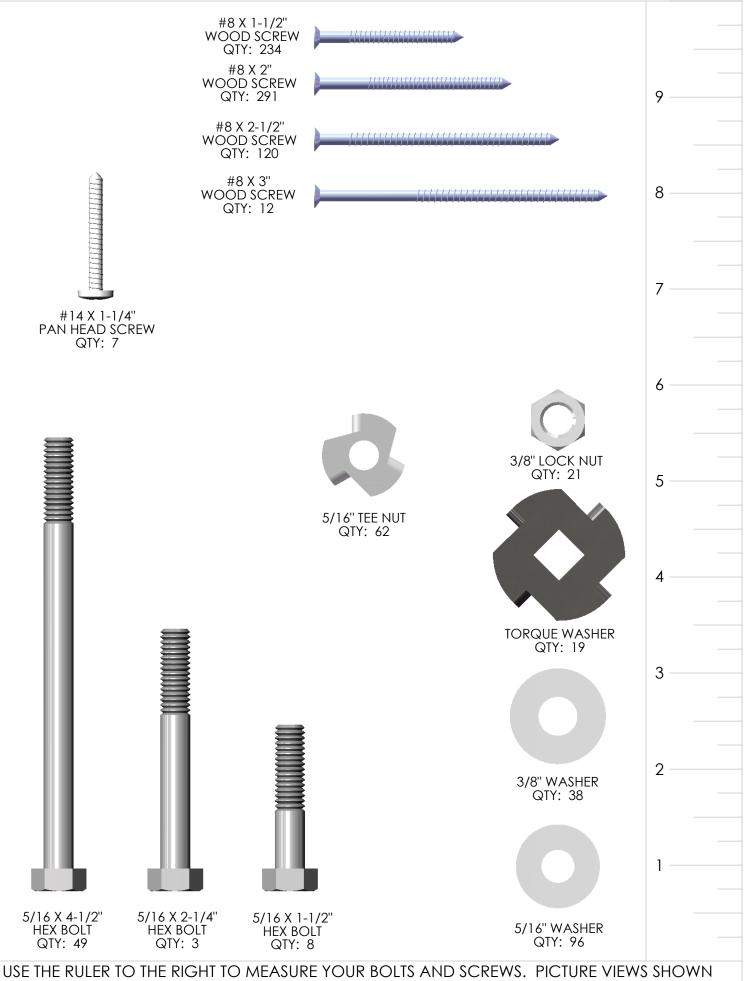
ABOVE ARE 1:1 SCALE AND CAN BE USED TO MATCH BOLT AND SCREW SIZES.
