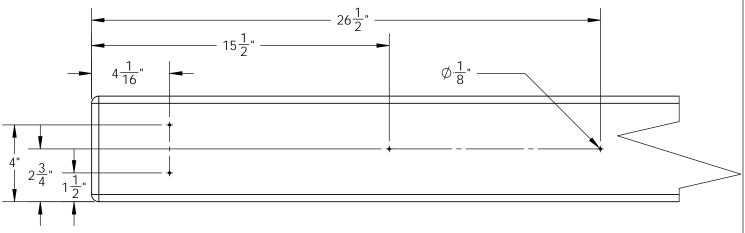
2: START WITH A 5/4 X 6 X 58" DECK BOARD AT ONE END OF THE FORT. CENTER THE BOARD BETWEEN THE REAR BOTTOM PANEL BOARDS AND LEAVE A UNIFORM SPACE BETWEEN THE DECK BOARDS. LAY ALL DECK BOARDS ACROSS THE DECK SUPPORTS BEFORE SECURING THEM TO THE FORT. THIS WILL ENSURE THAT YOU HAVE EQUAL SPACING ACROSS THE DECK.
