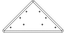
2: PLACE TWO OF THE 5/4 X 10" ROOF PEAK SUPPORTS AGAINST THE ANGLED ROOF SUPPORTS AND UNDERNEATH THE ROOF BOARDS. FASTEN THE ROOF PEAK SUPPORTS TO THE ANGLED ROOF SUPPORTS WITH 1-1/2" WOOD SCREWS.
