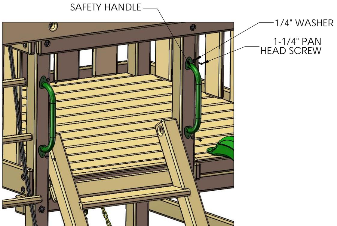
3: PLACE THE SAFETY HANDLES ABOVE THE BASE OF ROCK WALL ENTRY, CENTERED ON THE PANEL SLATS.
