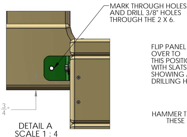
FLIP PANEL OVER TO THIS POSITION WITH SLATS SHOWING AFTER DRILLING HOLES
