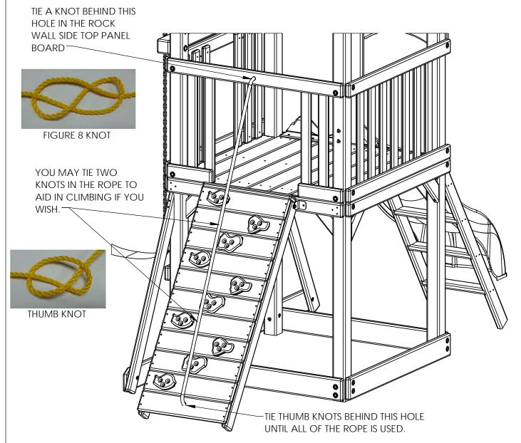
FOR SAFETY, ENSURE THAT THE ROPE IS TIGHT ENOUGH SO THAT IT CANNOT BE LOOPED BACK ON ITSELF.
