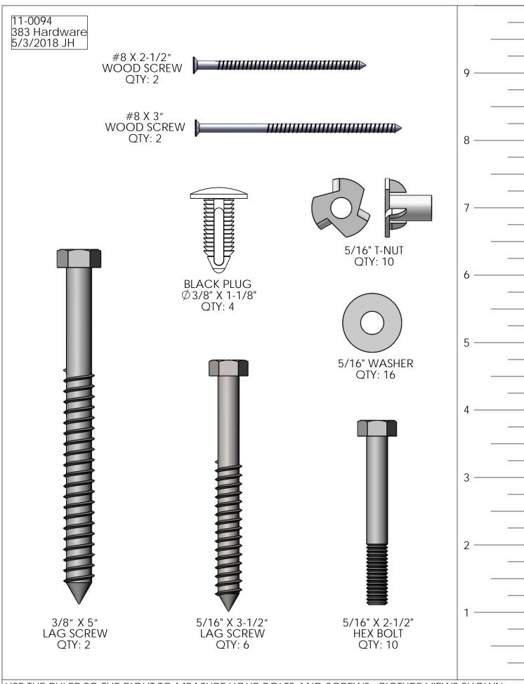
USE THE RULER TO THE RIGHT TO MEASURE YOUR BOLTS AND SCREWS. PICTURE VIEWS SHOWN ABOVE ARE 1:1 SCALE AND CAN BE USED TO MATCH BOLT AND SCREW SIZES.
