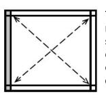
The diagonal measurements should be the same from corner post to corner post. If not, adjust corner posts so that the distance is equal.
