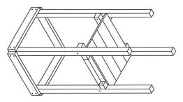
STEP 7 - PLACE THE 29 3/4 " DECK SPACERS (1) ON TOP OF THE DECK SUPPORTS, BETWEEN THE CORNER POSTS. FASTEN THE DECK SPACERS TO THE DECK SUPPORTS WITH WOOD SCREWS.
