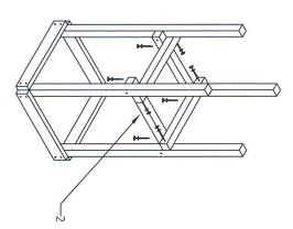
STEP 6 - PLACE THE 22 1/2 "BLOCKS (1) ON TOP OF THE BLOCK SUPPORTS, BETWEEN THE DECK SUPPORTS. FASTEN THE BLOCKS TO THE BLOCK SUPPORTS WITH 5 "LAG SCREWS W/ WASHERS.
