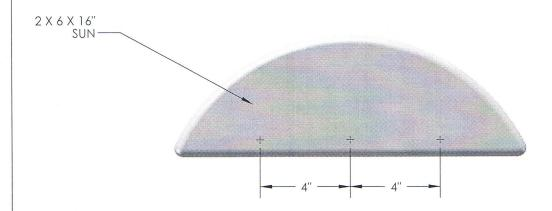
2: PLACE THE 2 X 6 X 16" SUN CENTERED AGAINST THE 5/4 X 2-5/8 X 42" SUN SUPPORT. FASTEN THE SUN TO THE SUN SUPPORT WITH 2" WOOD SCREWS. REPEAT THIS PROCESS FOR THE OTHER SIDE OF THE FORT.
