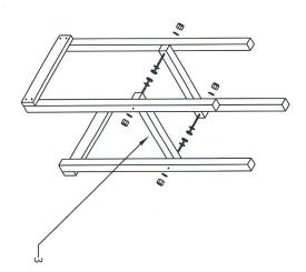
STEP 3 - PLACE THE REMAINING 36 3/4 " SAND BOX BOARDS (1) FLUSH WITH THE BOTTOM OF THE CORNER POSTS. FASTEN THE SAND BOX BOARDS TO THE CORNER POSTS WITH 3 1/2 " LAG SCREWS W/ WASHERS.
