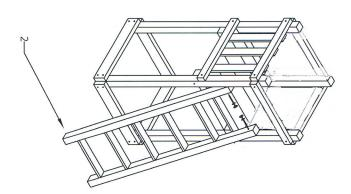
STEP 12 - PLACE THE 79 " SAFETY RAILS (1) FLUSH WITH THE INSIDE OF BACK CORNER POSTS OF THE THE FORT AND THE INSIDE OF THE FRONT CORNER POSTS OF THE TOWER, ALLOWING THE SAFETY RAIL TO REST ON TOP OF THE DECK OF THE TOWER. MAKE SURE THE SAFETY RAIL IS LEVEL. FASTEN THE SAFETY RAIL TO THE CORNER POSTS WITH 3 1/2 "LAG SCREWS W/WASHERS.
