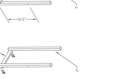
STEP 2 - PLACE THE 36 3/4 " BLOCK SUPPORTS (3) FLUSH AGAINST THE CORNER POSTS, LINING UP THE PILOT HOLES. FASTEN THE BLOCK SUPPORTS TO THE CORNER POSTS WITH 6 1/2 " CARRIAGE BOLTS W/ WASHERS.
