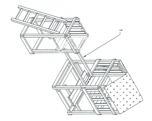
STEP 13 - PLACE THE 79 " SAFETY RAILS (1) FLUSH WITH THE INSIDE OF BACK CORNER POSTS OF THE THE FORT AND THE INSIDE OF THE FRONT CORNER POSTS OF THE TOWER. MAKE SURE THE SAFETY RAIL IS LEVEL. FASTEN THE SAFETY RAIL TO THE CORNER POSTS WITH 3 1/2 " LAG SCREWS W/ WASHERS.
