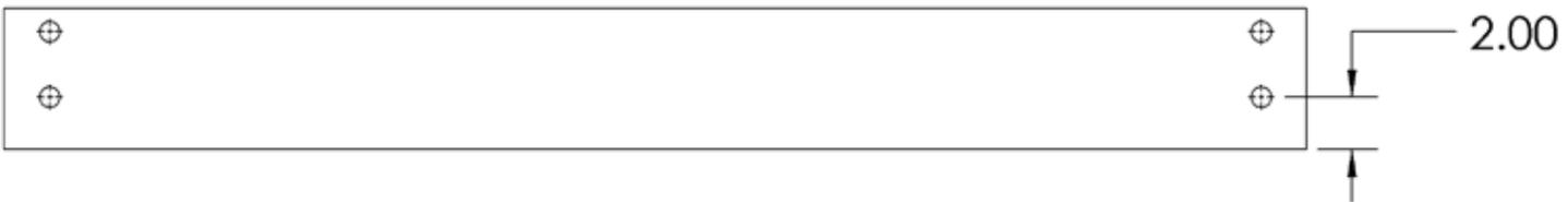
**Counter-sunk holes-** Many of the parts that will be used have counter-sunk holes. A counter-sunk hole is one that surrounds one side of a thru hole, but does not extend through the wood itself. When using a counter-sunk hole the bolt will be inserted through the thru hole. In some cases the bolt head with a washer will occupy the counter-sunk hole. In other cases a nut with a washer will occupy the counter-sunk hole.
