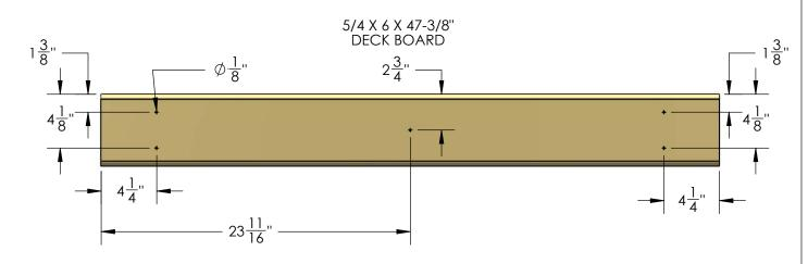
2: START WITH A 5/4 X 6 X 47-3/8" DECK BOARD AT ONE END OF THE FORT. CENTER THE BOARD BETWEEN THE FRONT DECK PANEL BOARD AND THE REAR DECK PANEL BOARD AND ATTACH IT WITH 2" WOOD SCREWS THROUGH THE PREDRILED HOLES AND INTO THE DECK SUPPORT BELOW. LEAVE A UNIFORM (APPROX. 1/4") SPACE BETWEEN THE DECK BOARDS. NOTE: THE TOP OF THE SCREW HEAD SHOULD BE FLUSH TO THE TOP OF THE DECK BOARDS.
