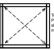
Top View of Playset Frame showing diagonal measurements. THE DIAGONAL MEASUREMENTS SHOULD BE THE SAME FROM CORNER POST TO CORNER POST. IF NOT, ADJUST FORT SO THAT THE DISTANCE IS EQUAL.
