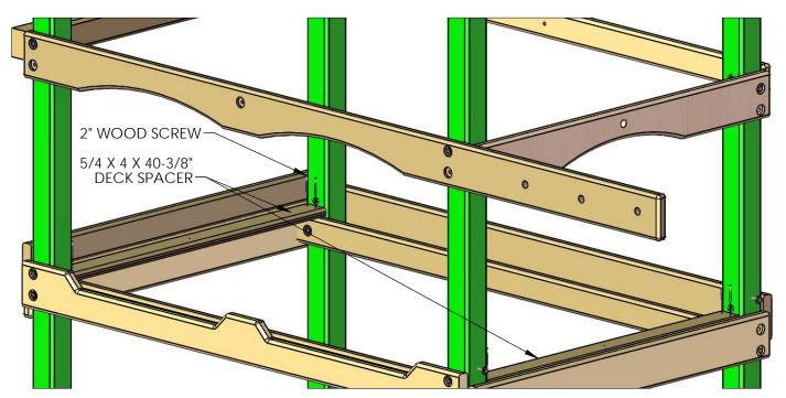
2 X 4 X 14" BOTTOM PANEL BOARDS REMOVED FROM VIEW FOR CLARITY
